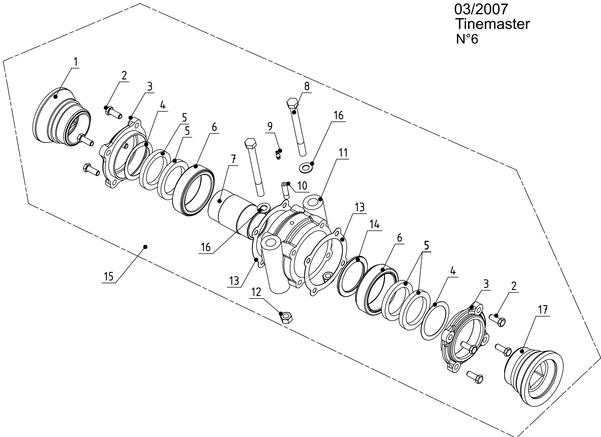
**5.20m and 6.00m Tinemaster front bearing assembly only**
