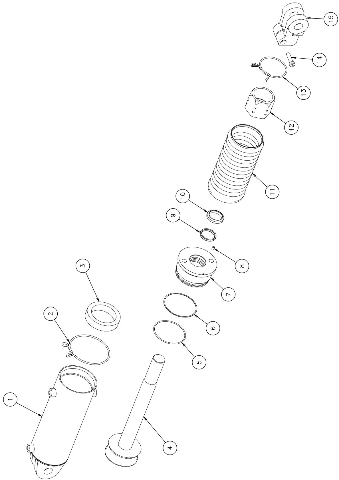
**1129      Hydraulic cylinder D100 x 200 mm w/stop and bellow
