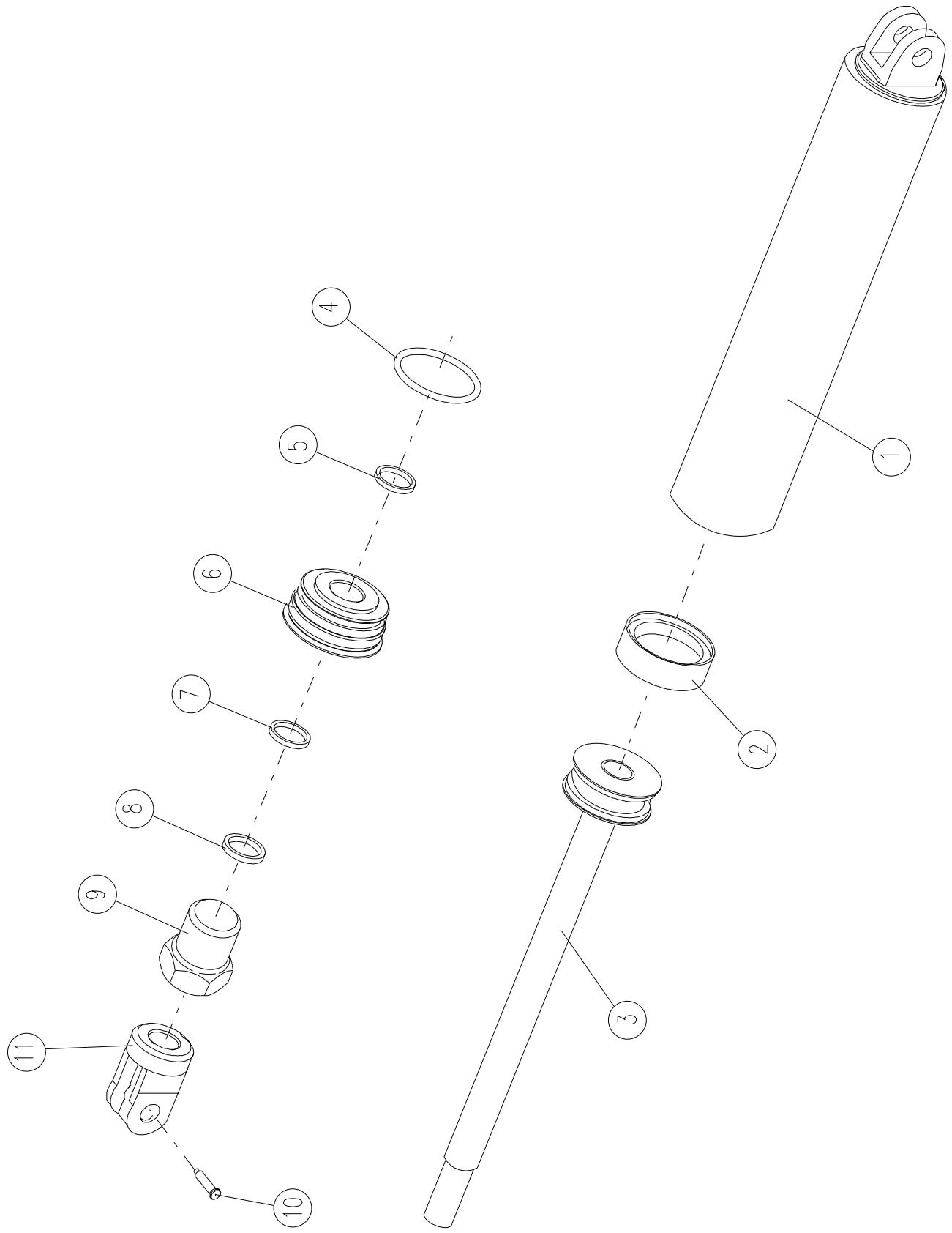
**1025      Hydraulic cylinder D75 x 400 and D100 x 400 mm w/stop
