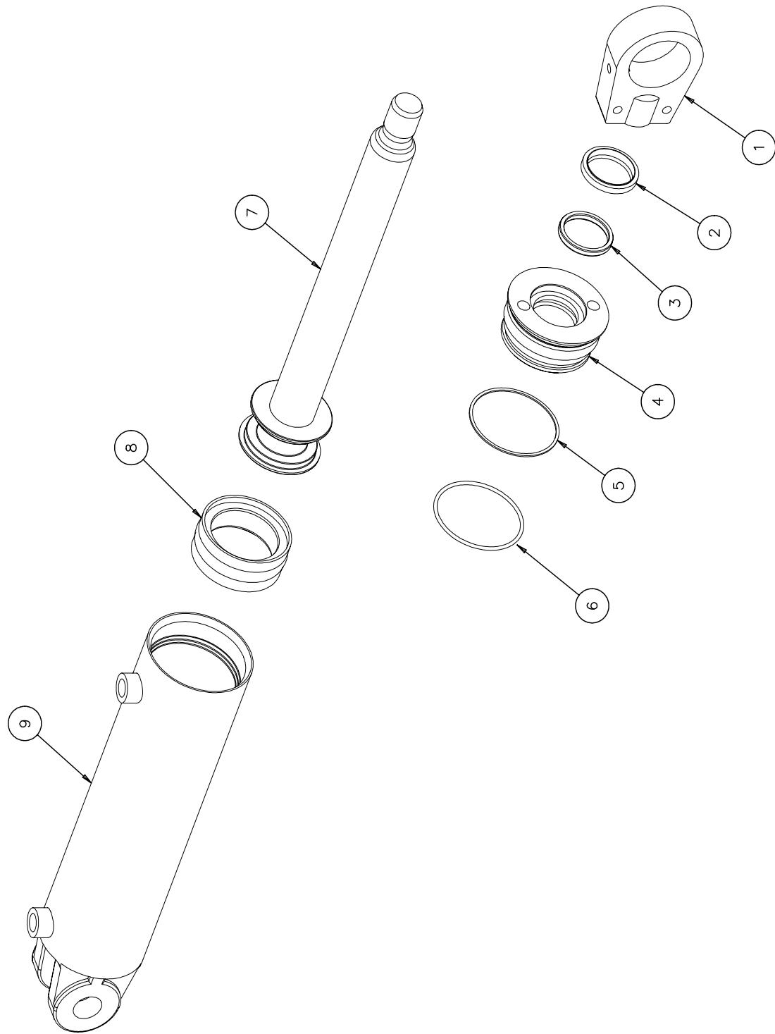
**1104      Support cylinder D80 x 240 mm**
