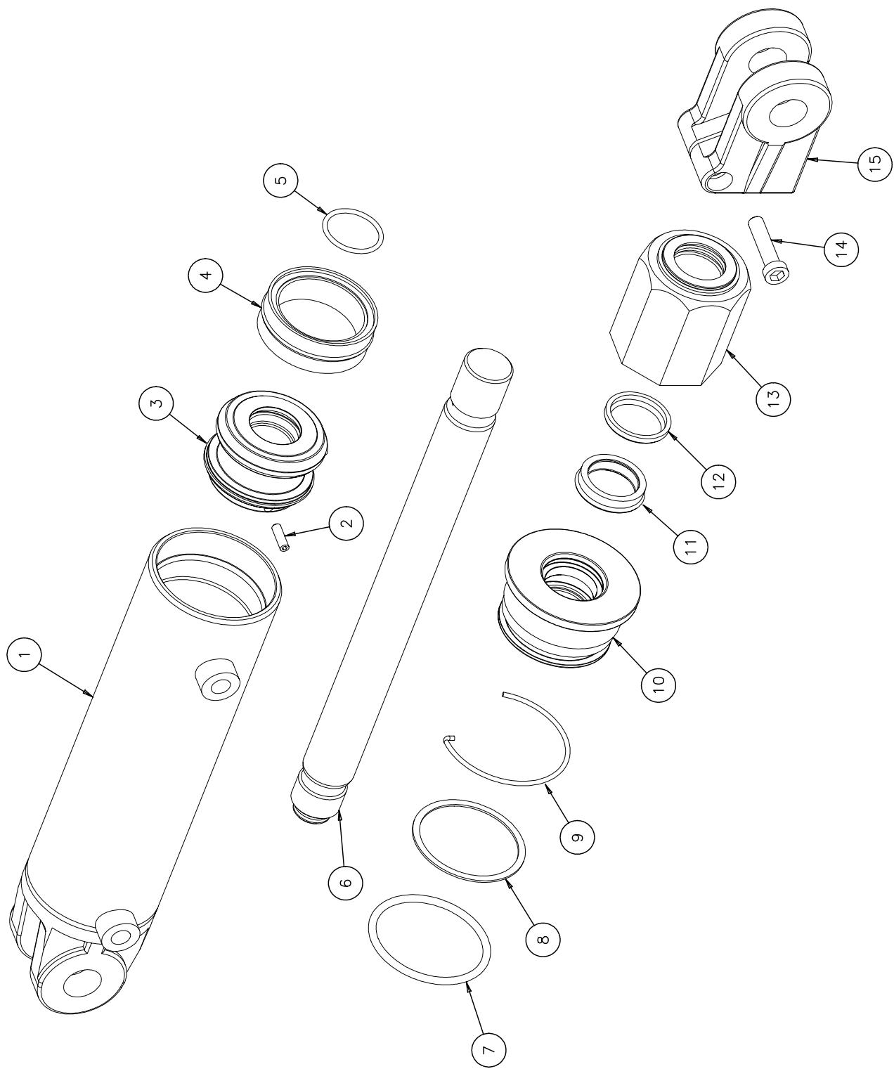
**890      Hydraulic cylinder D75 x 200 mm ( 353704 - 353707 )
