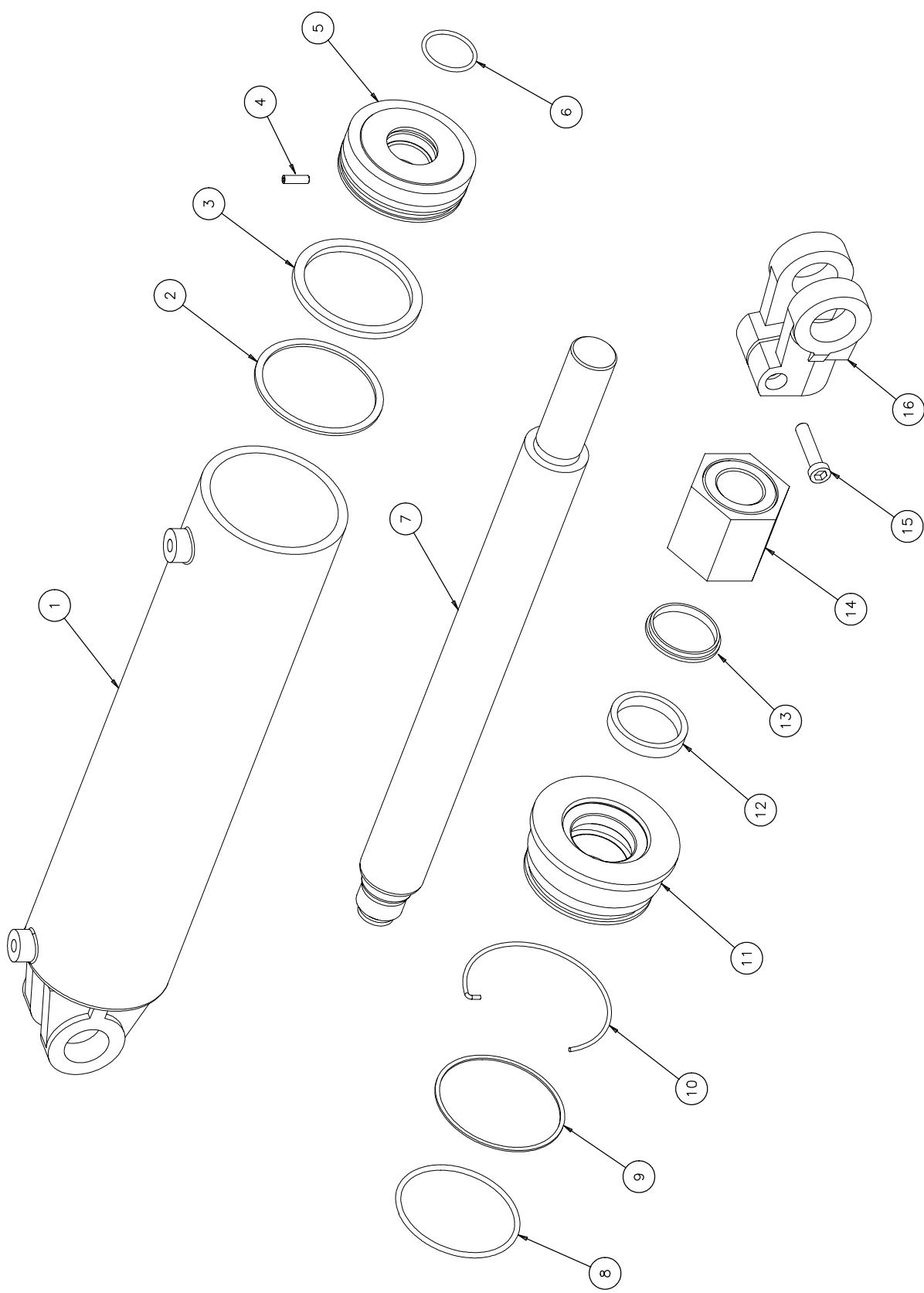
**1084 Hydraulic cylinder D100 x 400 mm w/stop ( From 15.05.99 )**
