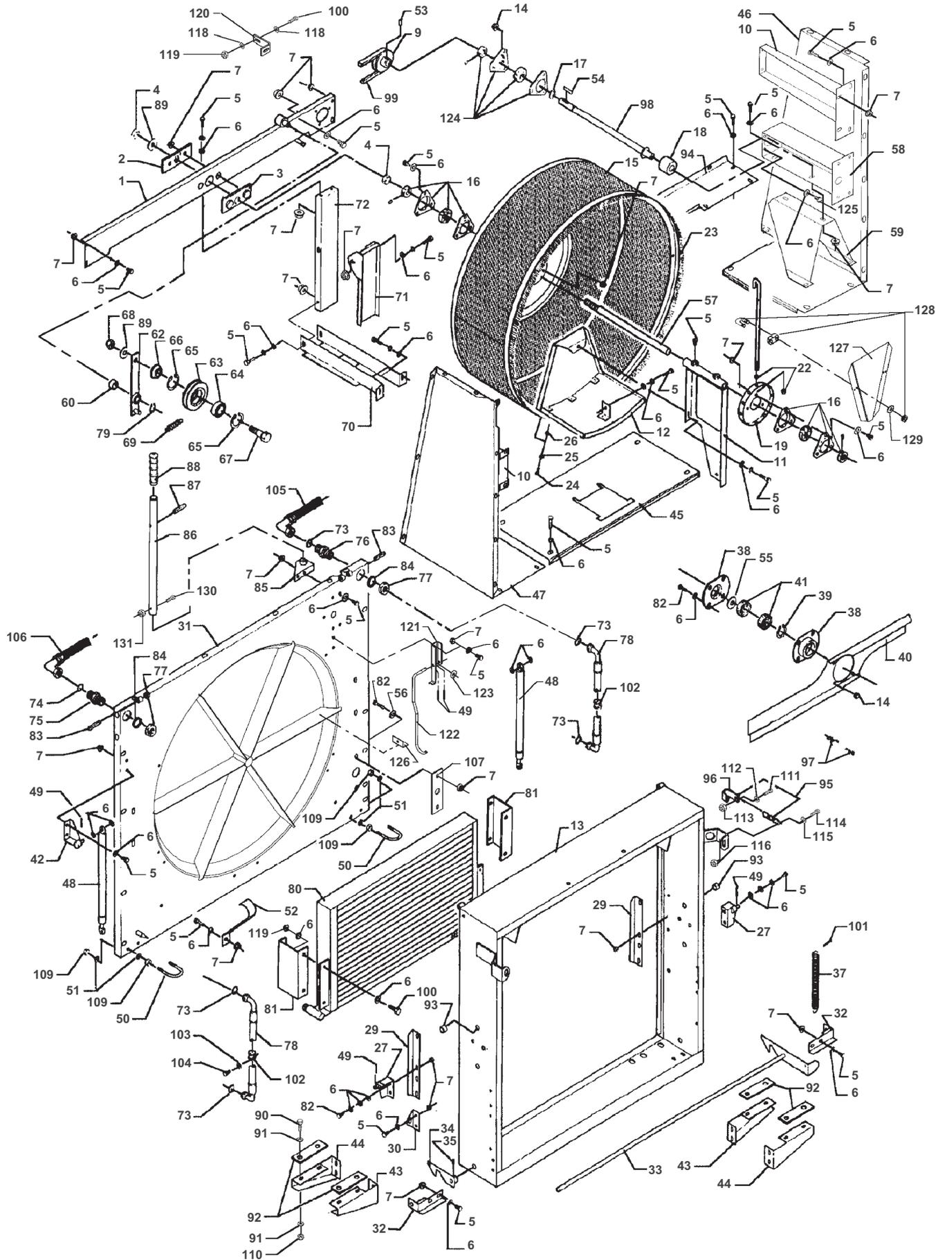
**Massey Ferguson****MF 38/40 COMBINES, |-> 47958 - 63001210****63001210****Rotary Screen - From Serial or Engine Number 48793****Page010-0020**
