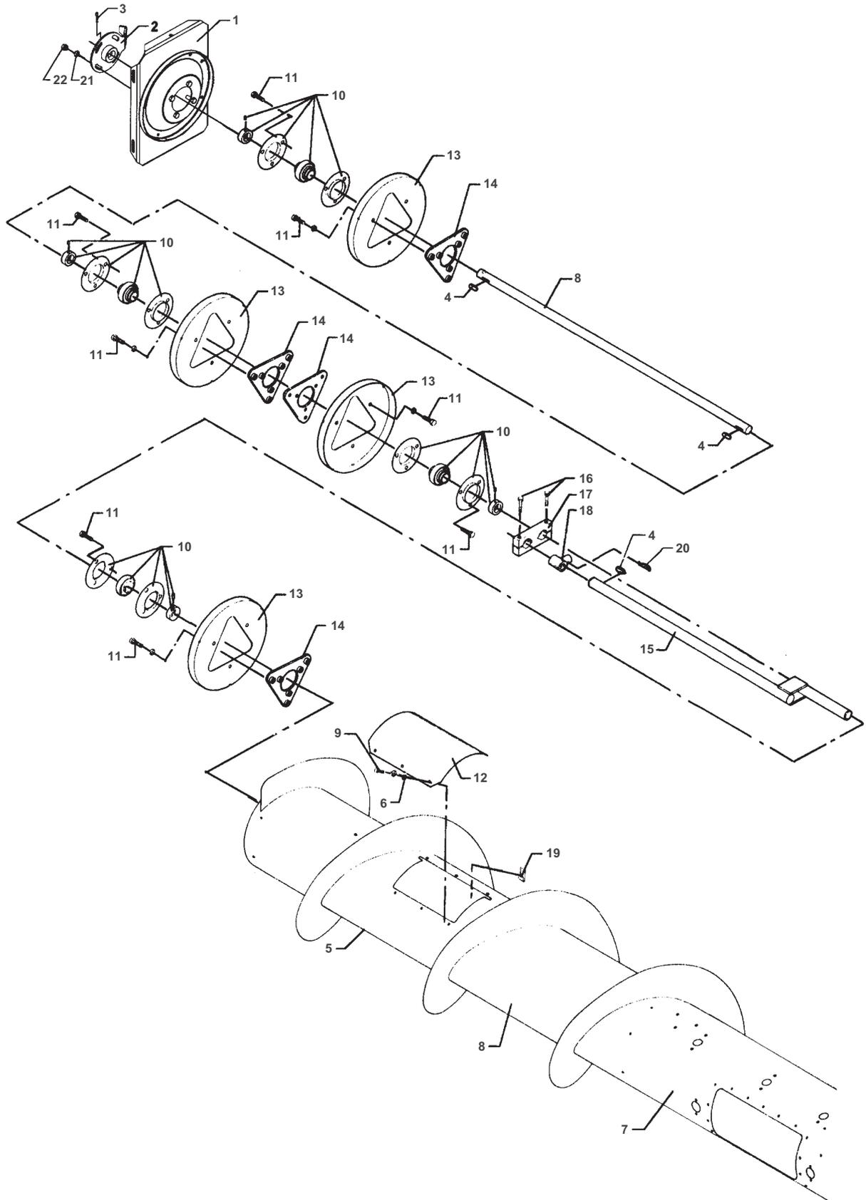
**Massey Ferguson****MF 38/40 COMBINES, |-> 47958 - 63001210****63001210****Feeder Drum Right Hand - Powerflow- - 7,80 M****Page001-0100**
