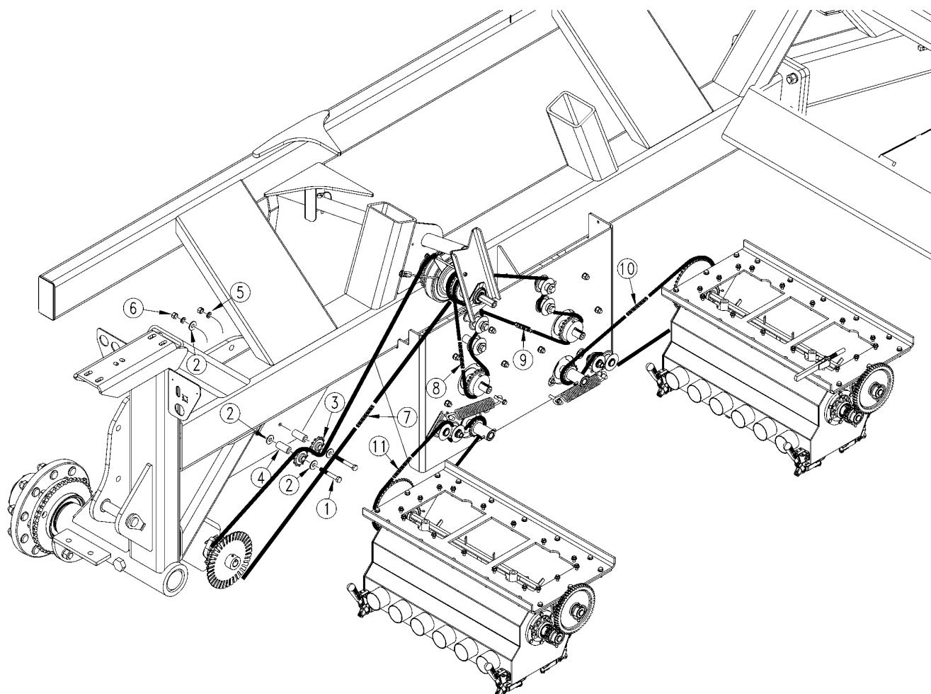
***Drive and Gearbox Chain Routing***
