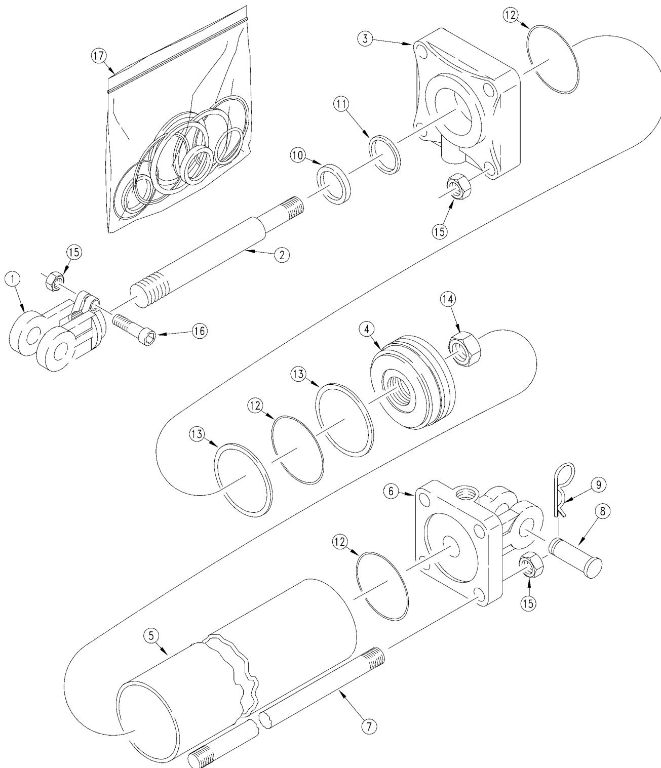
**Opener Lift Midway Hydraulic Cylinder 2 X 8 X 1.12 (810-299C)**
