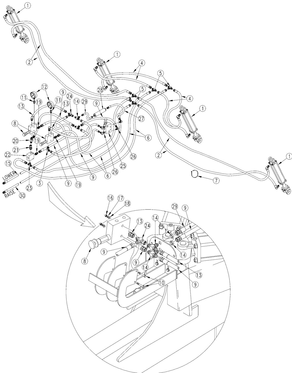
**Opener Down Pressure Hydraulics (Closed Center) (S/N DD1215-)**
