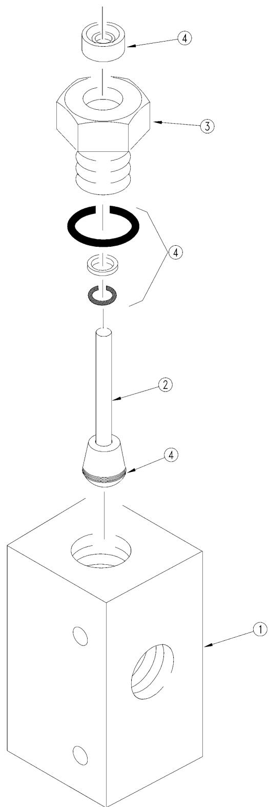
**Stroke Control Valve (810-445C)**
