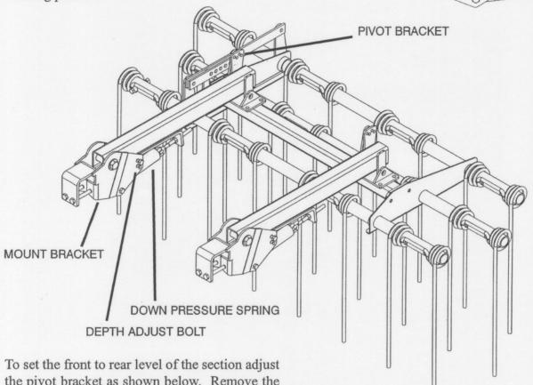
To set the front to rear level of the section adjust the pivot bracket as shown below. Remove the 1/2NCx1-1/2 GR5 bolts and rotate the section until the section is level. Reinstall bolts and tighten to specified torque.
